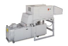
"Shredder baler combination for high security applications: equipped with a pre-shredder for 6 x 50 mm and an after-shredder for 2 x 4.5 mm cross-cut this shredder equals security level 4 according to DIN 32757 - compression in the integral baler in the next stage ensures that even the requirements of security class 5 can be fulfilled. Practical throughput of up to app. 150 kg per hour."
