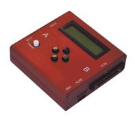
The intimus Hammer SE implements firmware-based erasure command to completely purge all data from parallel ATA (PATA) and serial ATA (SATA) hard drives.
